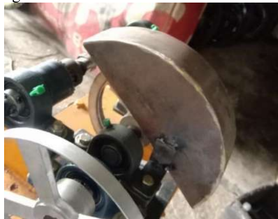
Gambar 4.19 Machine guard safety
